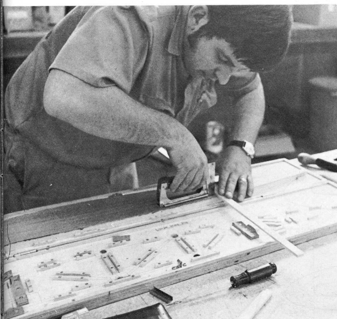
To insure uniformity, wing ribs are built in a jig. All jigs necessary for construction of the Acro Sport are shown in the plans.
